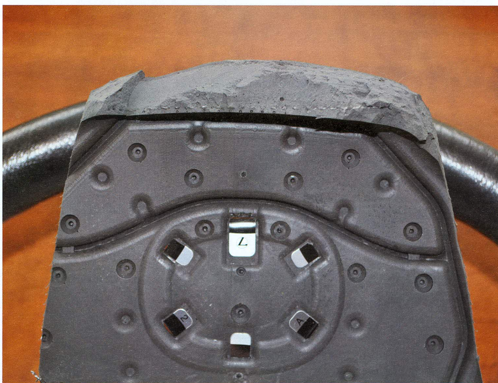
Figure 4. A view of the underside of the driver airbag door from the same airbag as shown in Figure 3. The bottom edge of the door (top of photo) is very roughly cut, and the airbag clearly did not deploy through the embossed seams that were moulded into the back side of the airbag cover, as designed. This airbag was also removed, tested and shown to be "live."
