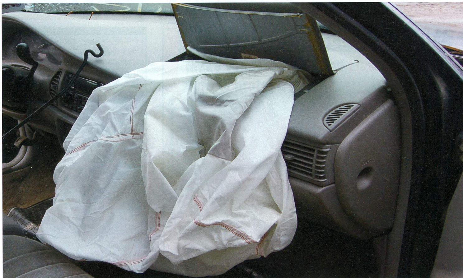
Figure 6. This vehicle was found with the airbags hanging out in the “deployed” condition, while the EDR recorded only a non-deployment event. The airbags were then removed and preserved for future testing.
