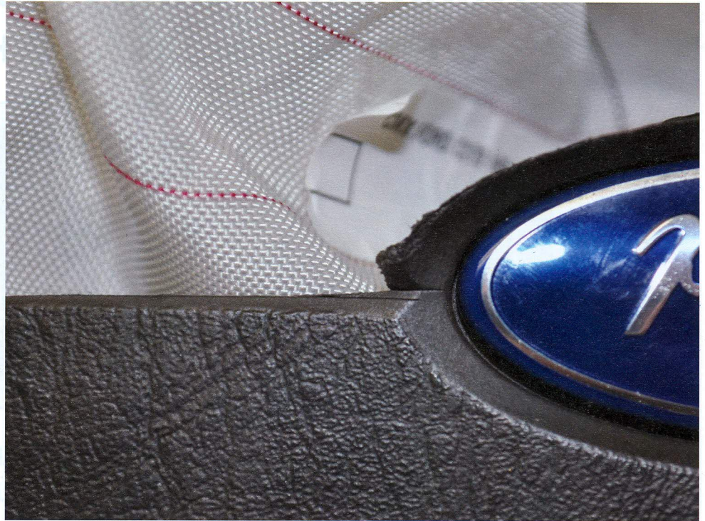
Figure 1. A close-up view of a driver airbag that was found in the "deployed" condition. The seams of the airbag door were very clean and sharp, and cut lines were evident leading to the centre emblem area. The airbag was removed, tested and found to still be "live."
