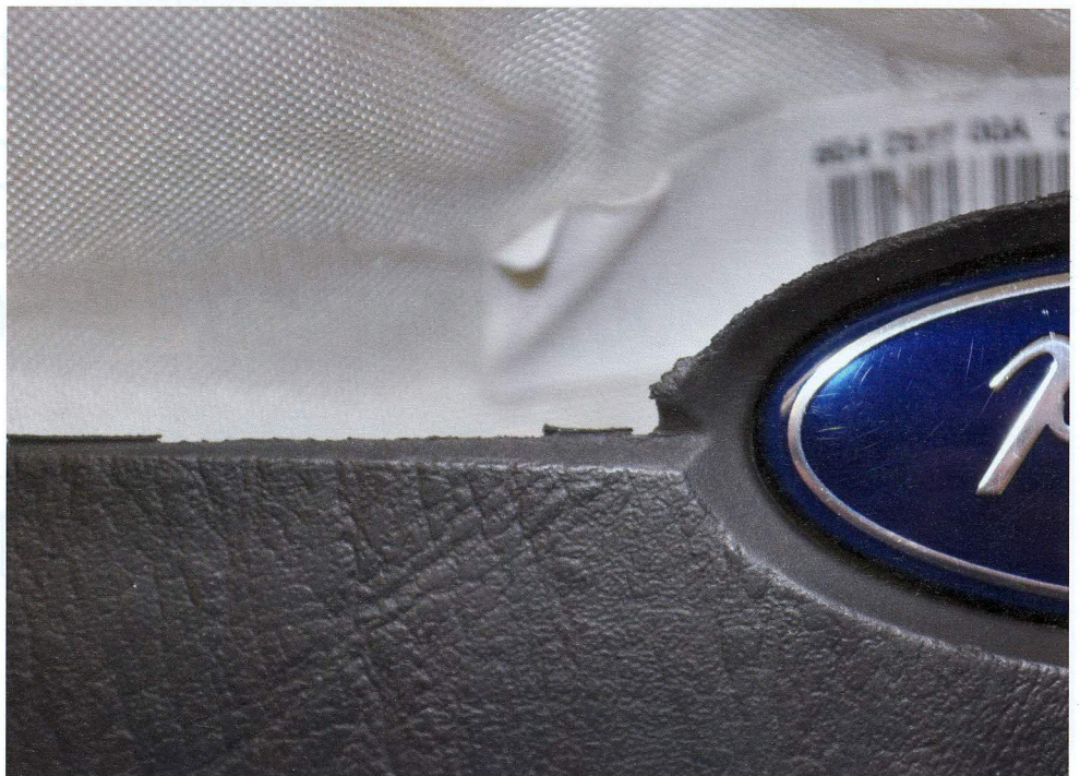
Figure 2. A close-up view of an airbag that was legitimately deployed in a controlled environment. The seam of the airbag door exhibited a slightly jagged appearance after deployment, and no cut lines were evident in the area around the centre emblem.
