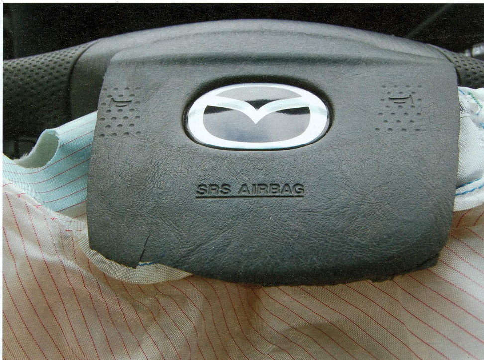
Figure 3. This driver airbag exhibited a very crudely cut airbag cover. Note the uneven profile along the bottom edge.
